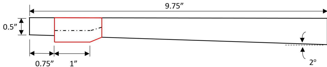
Figure 5.10: Thermally choked cavity combustor with heat release domain broken into 2 equal parts by the centerline. Each part will be modeled separately with equal heat release densities and compared.
